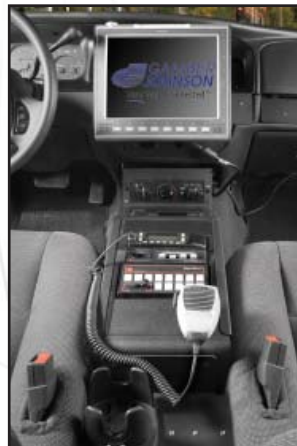
Low box installed in a Ford Crown Victoria
